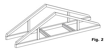
The 22" model is specially designed to fit between 24" on center truss ceilings. Install headers across truss cords to form a minimal 22" x 54" or 66" rough opening. Insure headers are plumb and square.
