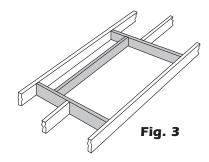
Installation parallel to existing joists normally requires a frame with single headers. (See Fig. 3)
