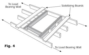
Installation perpendicular to the existing joists requires a frame with double headers (See Fig. 4). If joists must be cut, stabilize them by nailing 2 joist-size boards perpendicular to the ceiling joists before cutting. The double joist sections must be long enough to be supported by a load bearing wall at both ends.
