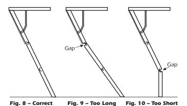
**Step 9–** Check to make sure of proper length. The stairs should fit flush with the floor and all joints should be tight with no gaps (Fig. 8 - 10).
