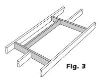
Installation parallel to existing joists normally requires a frame with single headers. (See Fig. 3)
