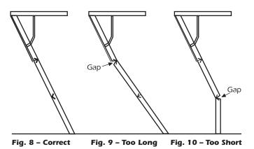
**Step 9–** Check to make sure of proper length. The stairs should fit flush with the floor and all joints should
