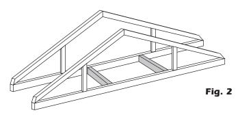
The 22" model is specially designed to fit between 24" on center truss ceilings. Install headers across truss cords to form a minimal 22" x 54" or 66" rough opening. Insure headers are plumb and square.
