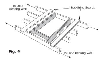
Installation perpendicular to the existing joists requires a frame with double headers (See Fig. 4). If joists must be cut, stabilize them by nailing 2 joist-size boards perpendicular to the ceiling joists before cutting. The double joist sections must be long enough to be supported by a load bearing wall at both ends.
