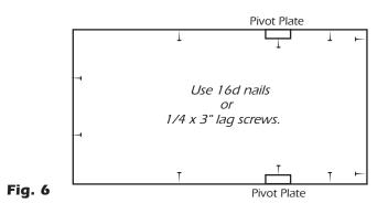
Holes have been predrilled in the pivot plates of the spring arms and the piano hinge. Also nail through the end board into the rough opening header. Complete permanent nailing with sufficient 16d nails to secure stair to all sides of the opening. Pilot holes should be drilled if lag screws are used. (See Fig. 6 above for suggested placement of nails.)
